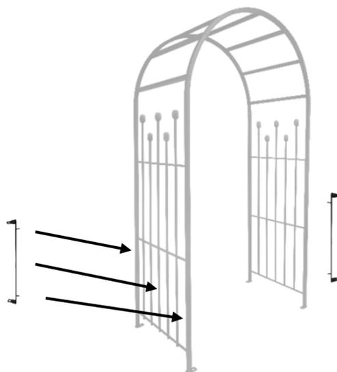
10. Place the connector bar in the desired position, secure with one bolt at the top end of the connector bar and one bolt at the bottom end of the connector bar.
