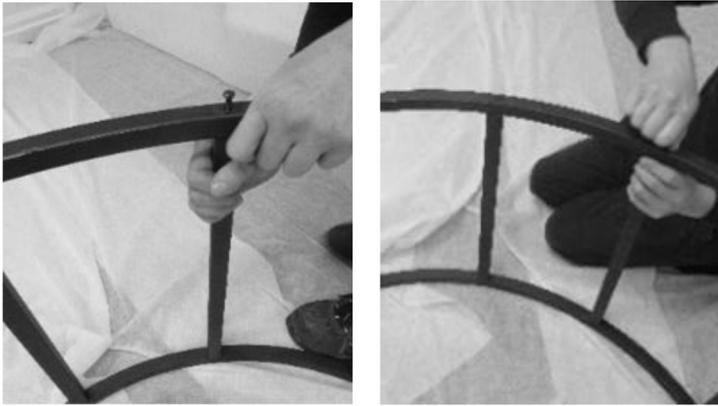
6. Slot one straight side piece into top curve with feet facing inwards.
