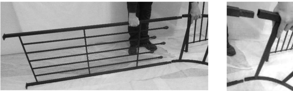
7. Slot the other straight side piece into the other side of the arch with feet facing inwards.
