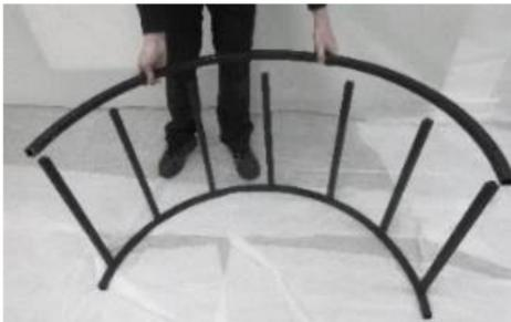
4. Attach the two outer cross beams to the second arched piece using long bolts.
