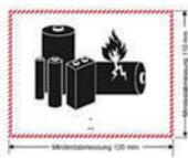
**Entry in AWB: LITHIUM ION BATTERIES in compliance with Section II of PI 965**
