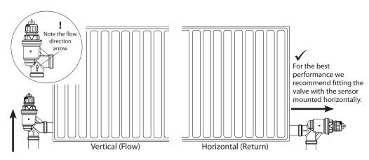
The Danfoss RAS-B<sup>2</sup> radiator valve can be fitted either vertically or horizontally.
