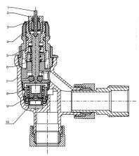
The thermostatic radiator valve consist of a sensor and the valve body RA-DV.
