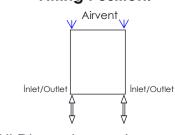
All Dimension are in mm Max.Working Pressure = 10 Bar Max.Working Temprature=95° C Inlet / Outlet : 1/2" BSP
