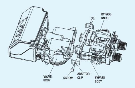
The bypass valve is provided with various functions such as bypass and water hardness adjustment.
