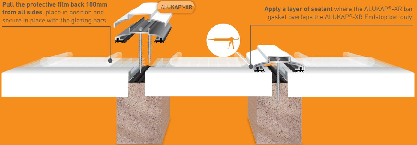
Apply a layer of sealant where the ALUKAP®-XR bar gasket overlaps the ALUKAP®-XR Endstop bar only.
