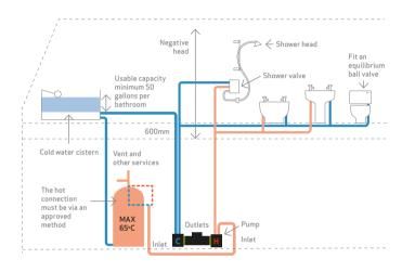
CT pump range twin ended universal to a bathroom in a loft conversion.
