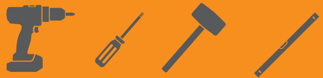
Cordless screwdriver/drill, Philips headed screwdriver, soft rubber headed hammer, a straight edge tool.
