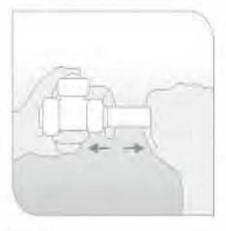
Press the demounting tool against the collet and then pull the pipe releasing it from the joint.
