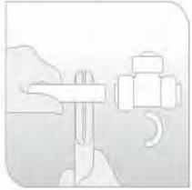
If the pipe is damaged (grab ring mark) while dismantling the fitting, then cut the pipe behind the grab ring mark to ensure the piece of pipe with the initial insertion is not reused.
