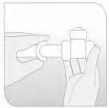
Ensure that the system is depressurized. Hold the pipe firmly and push the pipe inward toward the joint. Place the demounting tool against the collet.
