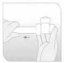
After checking the correct insertion depth has been achieved, pull back on the pipe firmly to ensure the grab ring engages correctly.
