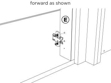
Ensure the hinge arm is at 90 degrees to the door before fixing in position with 15mm N screws as shown **B B** E
