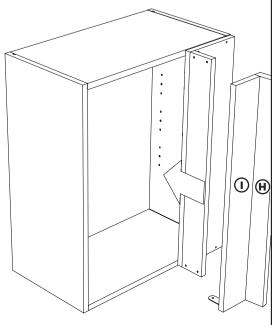
Attach corner post (I) to cabinet using brackets
