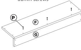
Align edges carefully and Screw blanking panels to assembled cabinet using 4 x
