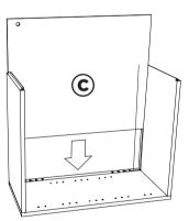
Press end panel A into top/bottom panels B and gently tap with a mallet
