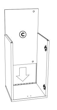
Press end panel A into top/bottom panels B and gently tap with a mallet
