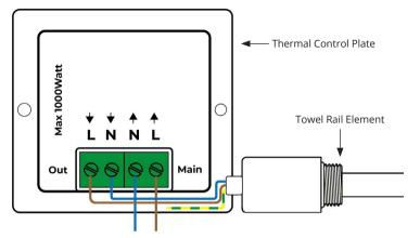
**Blue (neutral)** - to the 'N' marking on the 'OUT' side of the control plate.
