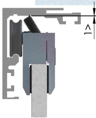
To prevent the hanger from rattling in the track tighten grub screw and leave a 1mm gap or smaller. Try not to obstruct the movement of the hangers.
