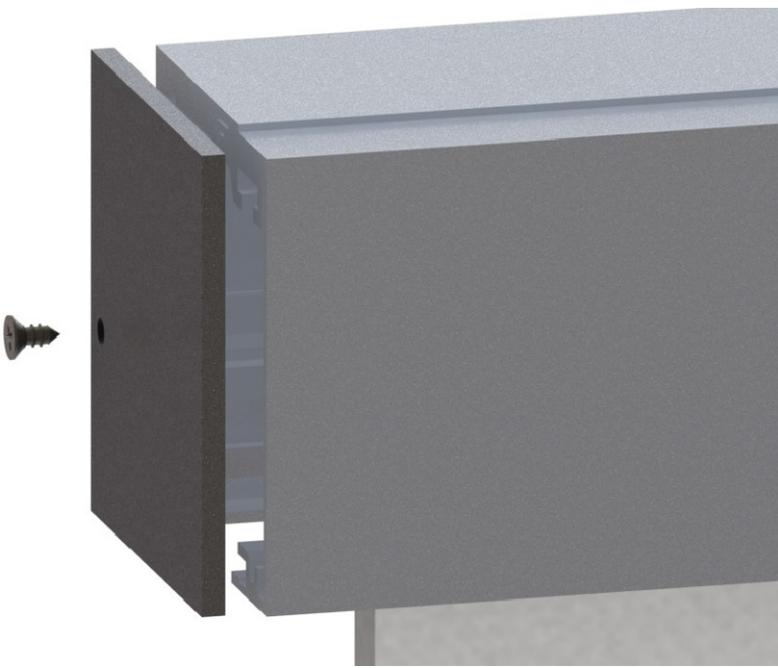
Put end caps into position and secure with screws
