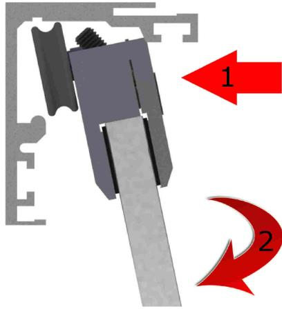
Adjust the height of the door by holding the **RED** nut with a spanner and rotate the **BLUE** grub screw with an allen key
