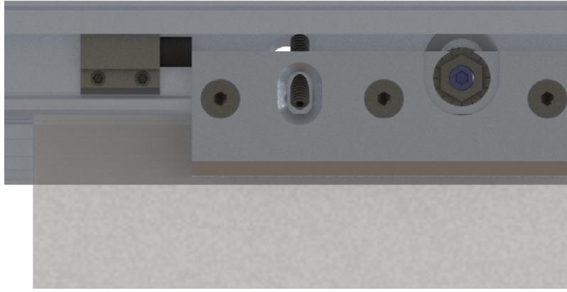
Insert stopper into track and secure it with screws
