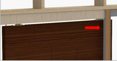
Slide the door inside the pocket to ease mounting the second door plate.
