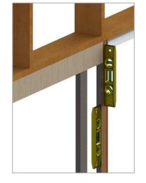
Ensure studs are straight (on the front and on the side). To double check if everything is straight the floor plate must be located in the middle of the chalk lines.
