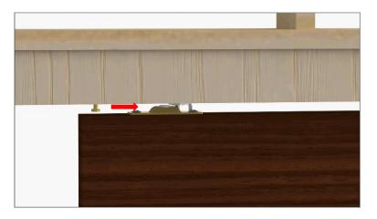
Insert hanger pin into the second door plate slot.
