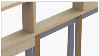
Fix the second pair of studs by butting them to the track equally spaced between the first set and the side stud, make sure they are in a levelled position and fix them with screws.
