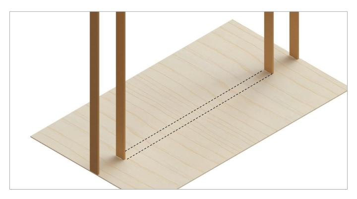
Make a straight chalk line on each side of the side studs to help define the pocket edges.
