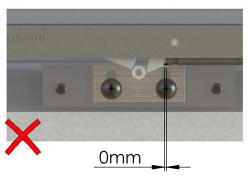
Insert the soft close stopper actuator into the soft closer head.
