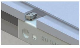
Fix the position of the soft closer by rotating the special nuts, which are located on each side of the soft closer
