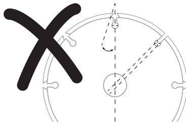
For all grinding, sanding, and wheel type wire brushing accessories, the lowest portion of the accessory must be contained within the guard enclosure with 2 mm or greater clearance to the bottom lip of guard.
