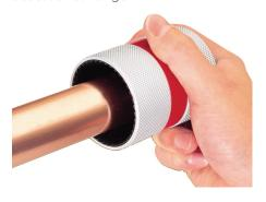
**3.** Clean the inside of the fitting socket and the outside of the tube with a Yorkshire cleaning pad, fine sandpaper or steel wool.
