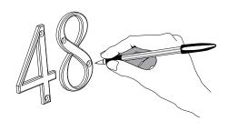
Remove the numerals. If available always use a drill punch to mark drilling positions using the pencil marks as a guide. The indent made by the point will ensure the drill does not slip.
