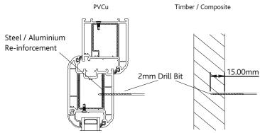
Align the numerals with thier correct fixing hole location. Screw into place using the correct screwdriver PH1 and using the fixing screws provided.
