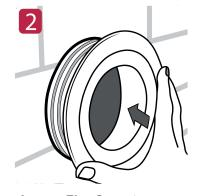
Insert FlueSnug into core-drilled hole
