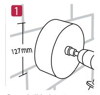
Core drill hole using standard 127mm core
