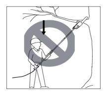
Never stand directly under the limb you are trimming. Always position yourself out of the path of falling debris.
