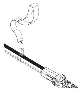
7. The telescopic shaft can be extended by releasing the lever (12) on the locking cam and extending the pole. Once the desired length is reached, lock the pole in position by closing the lever (12) on the locking cam. Ensure the pole is locked before using.
