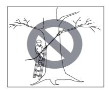
Never stand on a ladder or other type of unstable support while using the pole saw.
