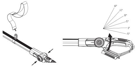
6. Assemble the strap belt (18) to the belt clip (17) on the pole and place over the shoulder added comfort.
