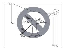
Do not use pole saw near cable, electric power or telephone lines. Maintain a minimum clearance of 3 metres from all power lines.
