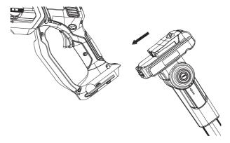
3. Slide the connection port slide lock to the on position (see below image), ensuring the shaft is securely fixed to the mini pruning chainsaw.
