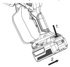
Align the battery port on the mini pruning chainsaw with the connection port on the telescopic pole. Slide the mini pruning chainsaw onto the connection port. It is successfully located into the connection port when you hear a click sound.
