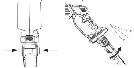
5. The handle can be set at 6 different angles and to adjust press the two angle adjustment buttons (11) and set at the required angle. To lock the handle in position, release the buttons and the handle will be set at the chosen angle.
