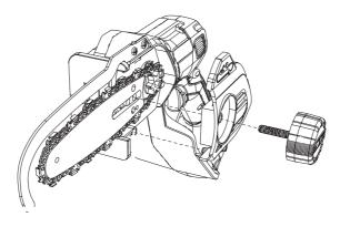
4. Use the hex key(6) attached on the chainsaw to adjust the chain tension by the chain tensioning hex screw(3)z showed in the figure below.
