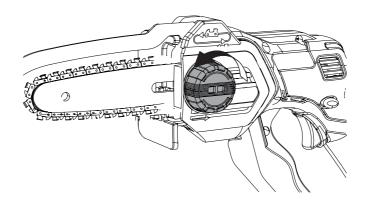
Hold the guide bar still and slide and wrap the chain in the groove around the guide bar. Ensure the chain tooth is in the correct running direction by comparing it to the chain icon on the guide bar and the machine.
