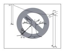
Keep other persons away from cutting end of pole saw and at a safe distance from work area.
