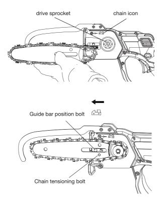
3. Replace the sprocket cover(5) onto the machine and insert the knob screw(9) into the middle hole of the sprocket cover(5). Turn the knob screw(9) clockwise to securely tighten the sprocket cover(5).
