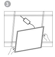
Fix the panel light into ceiling tile.
