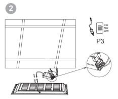
Feed the main AC wire in driver terminal block respectively, connect the panel light and driver.
