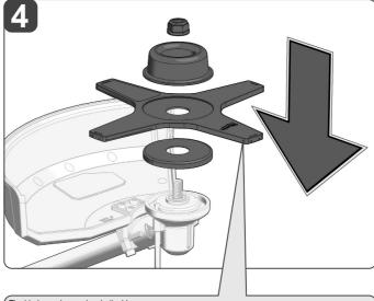
The blade can be used on both sides.
