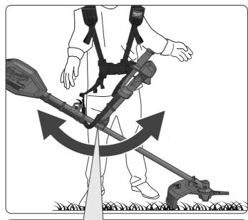
Level the appliance. The blade should touch lightly the ground.
