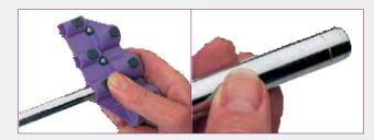
4. When jointing chrome-plated copper tube with Tectite Classic, Tectite Pro and Sprint fittings, scribe the tube using the T110/T115 (Sprint) scribing tool to ensure positive grab ring location. This helps to accommodate any variance in chrome plate thickness. Note: The scribing function is not suitable for stainless steel tube.
