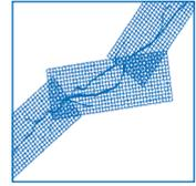
Square edge, butt or end joints should be finished approx 600mm wide.
