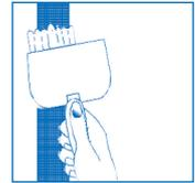
Continue along the length of the crack, ensuring complete and even coverage across the tape. Feather out beyond the taped edges by at least 50mm (the wider you finish the easier it is to disguise the repaired crack). Finish with a wet knife or allow to dry and sand. More than one coat may be required. If so finish at least 50mm beyond the previous coats.
