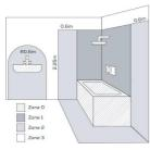
Suitable for indoor only. This product is rated as IP24. If the product is to be installed within a bathroom it can only be located within zone 2.
