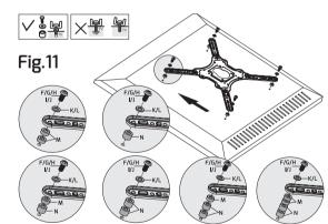
You can increase the spacing between the mounting plate and the back of the TV by using the spacers  $\emptyset/\emptyset$  see Fig.11.
