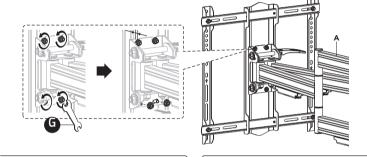
Lift and remove the VESA bracket as shown, keep the bottom nuts in a safe place.
