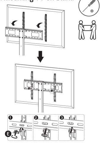
With two people, lift and hook the adaptor brackets onto the top and bottom of the plate. hold the TV in place, insert locking tabs • and tighten the bolts with a screwdriver to secure the adaptor bracket arms to the plate.
