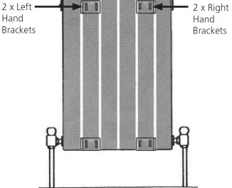
Aluminium radiators have specific left and right hand threaded bushes and these can be easily damaged if forced or incorrectly fitted (this will inevitably cause leaks). Bushes require a dry fit connection only; you must not use any Compound materials (e.g. Jet Blue) or Plumbers Hemp. If you choose you may use up to 4 turns of PTFE tape to help seal the threads (the tape should be applied in the direction of the thread and no more than this amount should be used as this may cause leaks to occur)
