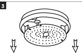
Carefully press and unlock the screw on the led hinged tray and hold the tray at an upward 90Degree position. Hold the product upside down.
