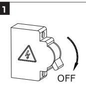
Switch OFF the power before starting the installation.
