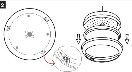
Remove the cover by holding the luminaire upside down. Press 3 clips on the sides and pull the base upwards to open and set aside.
