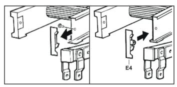
4.9 Locate the power arm linkage plates either side of pivot tip (E4)/ladder stile and align all holes.
