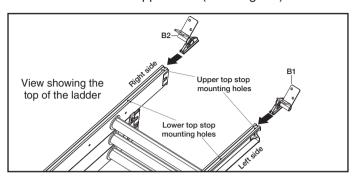
Slide the hinge guides past both sets of top stop mounting holes, so that the hinge guides are below the top stops, when they are fitted in section 2.
