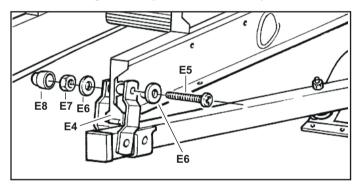
DO NOT over-tighten the nut as this will restrict smooth operation of the ladder system.
