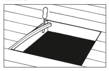
**I.4** Screw hinges (F5) to one edge of the trapdoor using 20mm (3/4") wood screws (F6).
