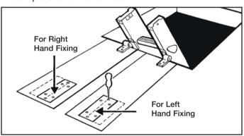
4.3 Place the spring housing (E1) in position over the holes ensuring the arm points AWAY from the loft opening (with slot in cover on the left-hand side).
