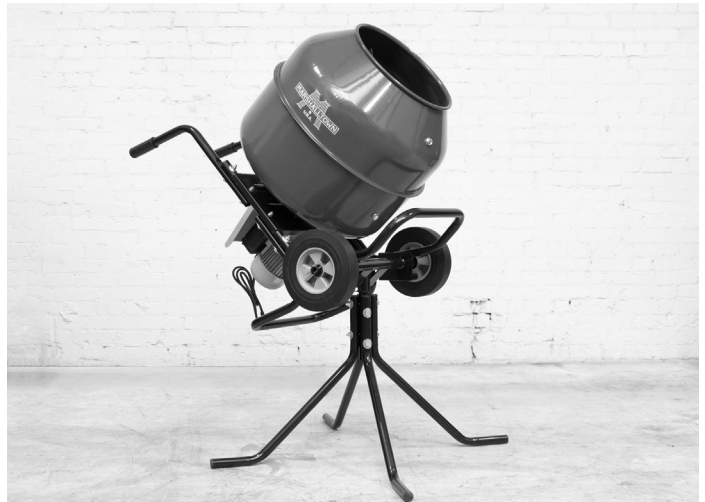
Completed mixer with pedestal.
