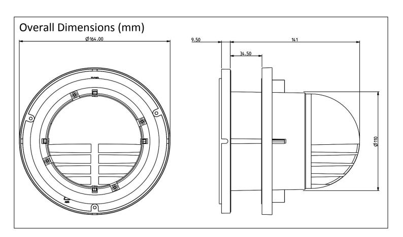
Kit must be installed with slots orientated downwards as shown
