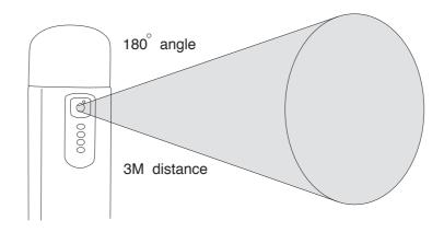
The PIR economy feature enables the outdoor heater to automatically shut down its heating function when not in use. The PIR sensor constantly monitors peoples movements up to a distance of 3 metres and if after 4 minutes it does not detect movement it will switch the heating off. The heating won't be on afterwards unless you operate from the panel or the remote controller.
