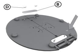
1 Align the two halves of the Base(L), make sure the wheel and axle are in position. Insert bolts with washers (Ex4+Cx4).
