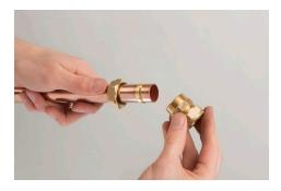
Remove the compression nut and compression olive, then put the nut on the tube, followed by the olive. Insert the tube end up to the fitting's tube stop. Slide the olive and the nut down to the fitting body. Tighten the nut using your fingers to secure the fitting in place.
