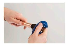
Using your deburring tool, make sure the inside of the pipe is smooth and will not interfere with the flow.
