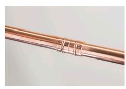
You should allow the joint to cool naturally. Cooling the joint forcefully could stress the joint.
