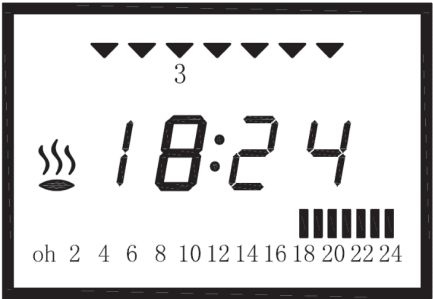
Example display after setting: Wed., timer setting from 18:00 to 24:00
